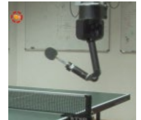
Figure 5: Sketch of SARCOS anthropomorphic robot arm
